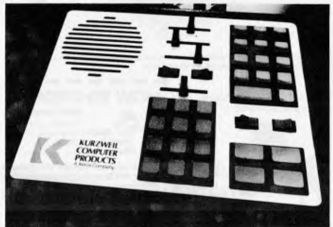
Kurzweil Reading Machine control panel. Type converted to speech
